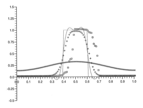
Figure 3: Constant advection after ten rotations. Exact and exactly integrated Lagrange-Galerkin solutions—solid lines, Monotone (Simpson's rule)— $\square$ , Van Leer's limiter—+, lumped scheme—×.  $\Delta x = 1/100, \ \nu = 5/12.$
