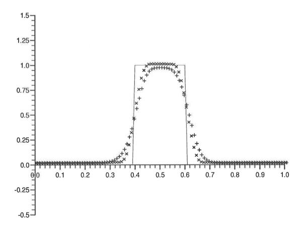
Figure 4: Constant advection after ten rotations. Exact solution—solid line, Monotone (Exact Integration)— $\times$ , Van Leer's limiter—+.  $\Delta x=1/100,\ \nu=5/12.$
