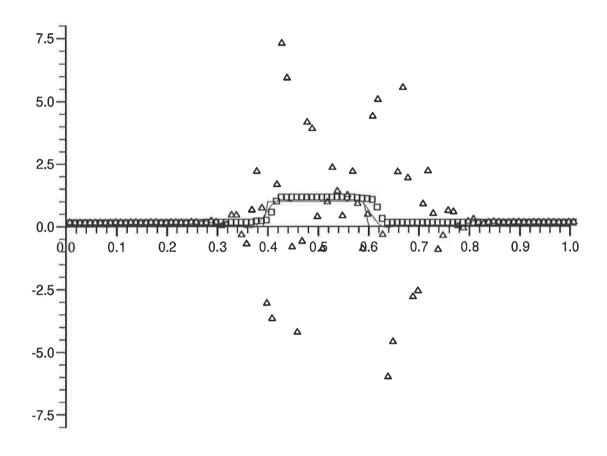
Figure 2: Constant advection after one rotation. Exact and exactly integrated Lagrange-Galerkin solutions—solid lines, Simpson's rule— $\triangle$ , Monotone (Simpson's rule)— $\square$ .  $\Delta x = 1/100$ ,  $\nu = 5/12$ .
