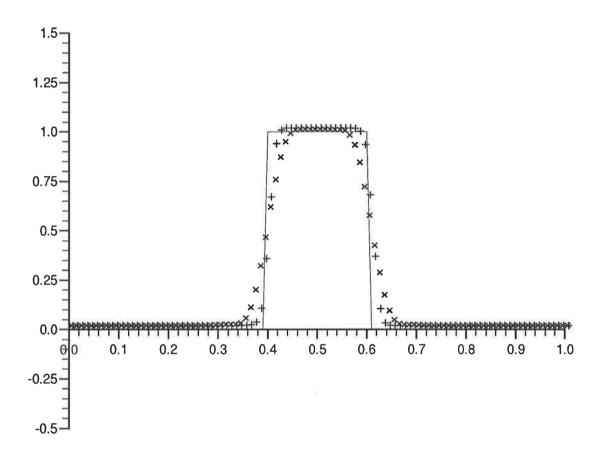
Figure 5: Constant advection after ten rotations. Exact solution—solid line, Monotone (Exact Integration)— $\times$ , Superbee limiter—+.  $\Delta x = 1/100$ ,  $\nu = 5/12$ .
