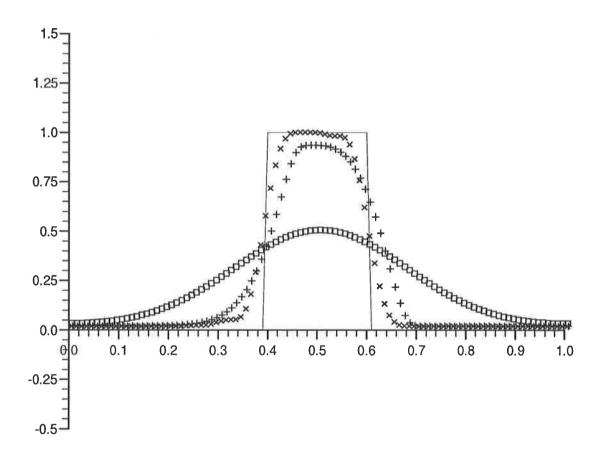
Figure 6: Constant advection after ten rotations. Exact solution—solid line, Monotone (Exact Integration)— $\times$ , Monotone (Simpson's rule)— $\square$ , Van Leer's limiter—+.  $\Delta x = 1/100, \ \nu = 1/12.$
