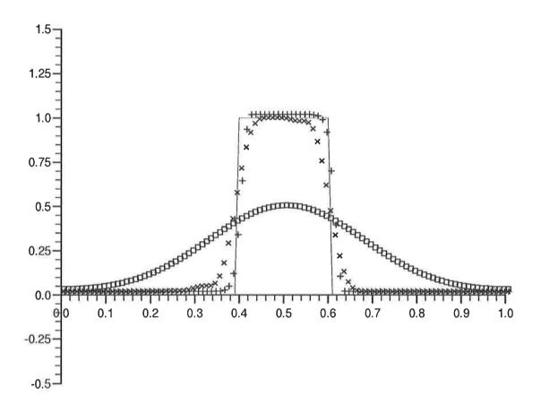
Figure 7: Constant advection after ten rotations. Exact solution—solid line, Monotone (Exact Integration)— $\times$ , Monotone (Simpson's rule)— $\square$ , Superbee limiter—+.  $\Delta x = 1/100$ ,  $\nu = 1/12$ .
