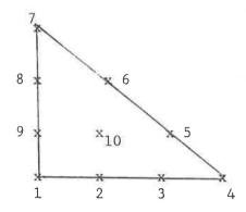
The transformation of the general 10-noded cubic triangle on to the standard triangle is defined by:
